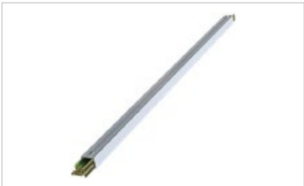
E SERIES DECKING BEAM Adjustable length – 2.33mtrs to 2.61mtrs Working limit shoring 1000kg 1500kg (evenly distributed fixed load).
